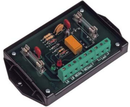
The APU-1B is for 120 VAC applications, while the APU-1C is for 208-277 VAC applications. The application for the APU-1x is metering configurations where dual service is provided to the customer, but meter potentials are only on one service. To insure that the meter is always energized and measuring energy use, the APU-1x switches from the primary source to the auxiliary source if the primary source is lost.
