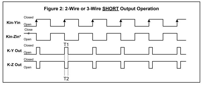
If the input pulse rate is greater than 9 pulses per second or if pulses of 100mS are too short for the receiving equipment, it is recommended that the <u>LONG</u> pulse output mode be used. Contact the factory for technical support at (888)272-9336.
