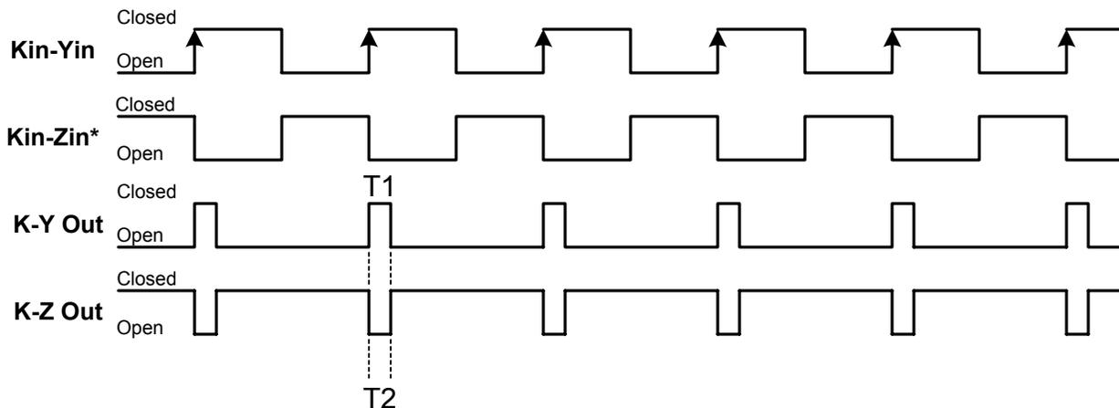
If the input pulse rate is greater than 9 pulses per second or if pulses of 100mS are too short for the receiving equipment, it is recommended that the LONG pulse output mode be used. Contact the factory for technical support at (888)272-9336.
