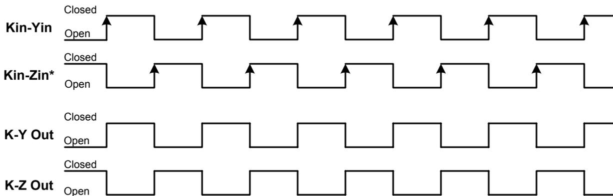
In the Short output mode, shown in Figure 2 below, an output pulse (K-Y closure) with a fixed width (T1) of 100mS occurs each time the input is triggered. Correspondingly, the K-Z output opens for 100mS (T2) each time the input is triggered. In the "short" mode, the output pulse rate is limited to about 9 pulses per second, or about 32,400 pulses per hour.
