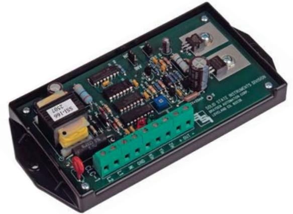
scaling of interpretation of a value of a pulse. The output can be configured so that a K-Y closure will result in either 4mA or 20mA. Once set, the K-Z closure becomes the opposite milliamp output. In this way, a KYZ pulse output can be configured to interface directly to a process control system or other instrumentation with a 4-20mA input.
