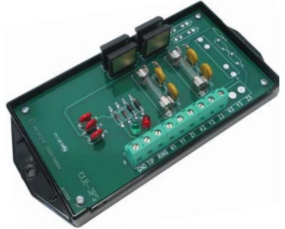
Applications include long distance pulse transmission interfaces up to 2-4 miles between utility metering devices and customer-owned energy control systems, demand recorders, or supervisory control (SCADA) systems.
