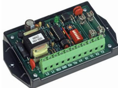
The DPR-4 microcontroller checks the input pulse for valid timing, and counts the input pulses for division only when valid pulses occur, thus assuring a high degree of noise rejection. Bright red and green LED lamps indicate the input and output status, respectively, all times thus allowing a rapid visual check-out of the system's performance without requiring any additional test equipment.
