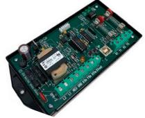
The DPR-2 is a programmable microcontroller-based, high-speed dividing pulse relay designed to provide two independent "dry" 2-wire Form A contacts (K & Y) from a 2-wire Form A pulse input. An output pulse occurs when a specified number of input pulses have been received. The divider's ratio of input to output pulses may be set between .00001 and 100,000. Using floating point math, the DPR-2 can be configured to scale input to output pulses to an exact ratio desired.
