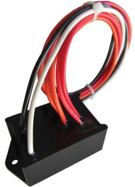
The LCR-4 is designed to provide isolation and improve safety and reliability when switching loads or control circuits involved in a load management program. A 2-wire, dry-contact output from the meter is used to activate the higher current output as shown in the figure below. It provides a very low-current sense wetting voltage and may be used with meters having a dry-contact output whether electro- mechanical, or high or low voltage semiconductor outputs.
