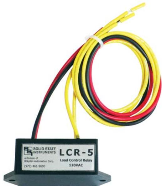
The LCR-5 is designed to safely interface with utility load management receivers, customer-owned equipment or control circuits involved in load management programs. A 2-wire, dry-contact output from the meter is used to activate the higher current output as shown in Figure 1 below. It provides a very low-current sense wetting voltage and may be used with meters having dry-contact outputs whether electro-mechanical, or high or low voltage semiconductor outputs.
