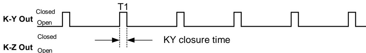
In Signed mode, with a Form A output mode selected, the K-Z output pulse represents negative (or *kWh Received*) energy. (See Page 6.)
