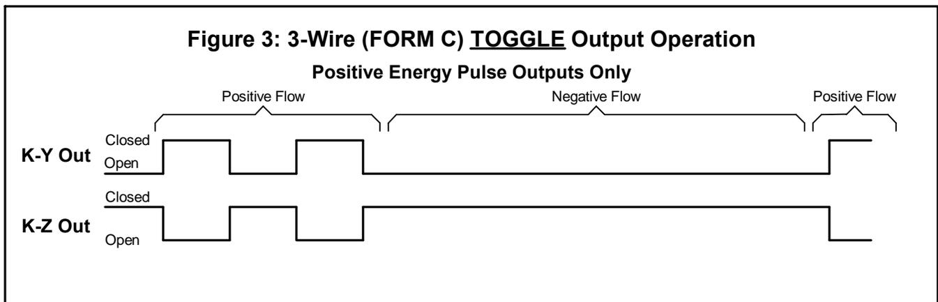
In Signed mode, with a Form C output mode selected, the K-Y and K-Z output pulses represent positive (or kWh Delivered) energy; Negative (or kWh Received) energy is ignored.
