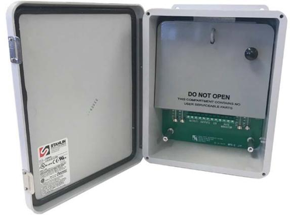
The MPG-2 features a USB input to host the Zigbee radio module “dongle” (included) and two KYZ pulse outputs. As the MPG-2 receives periodic usage data from utility's meter, the data is read and interpreted to obtain the current demand information. The accumulated energy is computed and pulses are outputted according to a selected pulse value.
