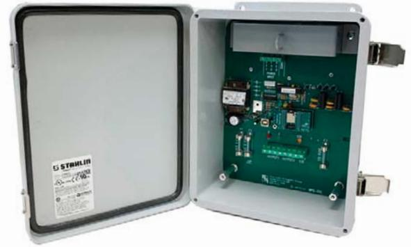
The MPG-3SC features integral Zigbee radio module and two KYZ pulse outputs, in a fiberglass NEMA 4X enclosure. As the MPG-3SC receives periodic data from utility's meter, the data is read and interpreted to obtain the current demand information. Accumulated energy is computed, and pulses are outputted according to a selected pulse value.
