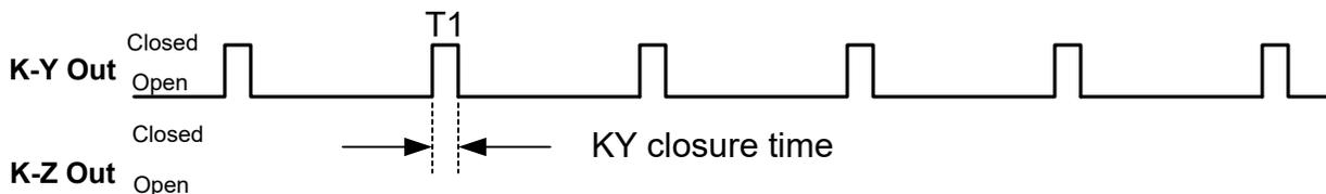
In Signed mode, with a Form A output mode selected, the K-Z output pulse represents negative (or kWh received) energy. (See Page 8.)
