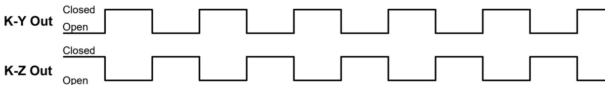
In the Fixed output mode, shown in Figure 2 below, an output pulse (K-Y closure only) is a fixed width (T1) each time the output is triggered. The pulse width (closure time) is determined by the setting of the W command. This mode is best for energy (kWh) counting systems but may not be the best for systems doing demand control where pulses are timed to derive instantaneous kW demand. The K-Z output is not used in the normal/fixed mode. However, it is used in the Signed mode. See Page 8.
