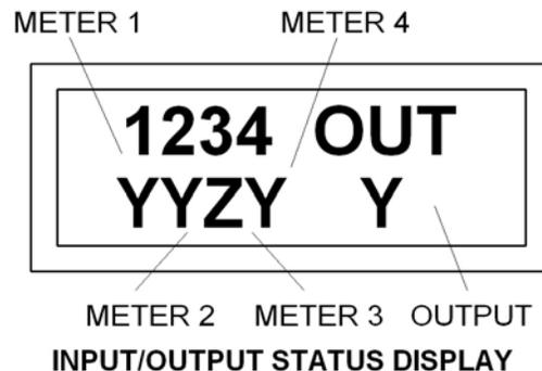
“K” and “Z” on the output are closed or “made up”. The “K” to “Y” output contacts are open. **PRESS THE ORANGE KEY TO GO TO NEXT DISPLAY.**
