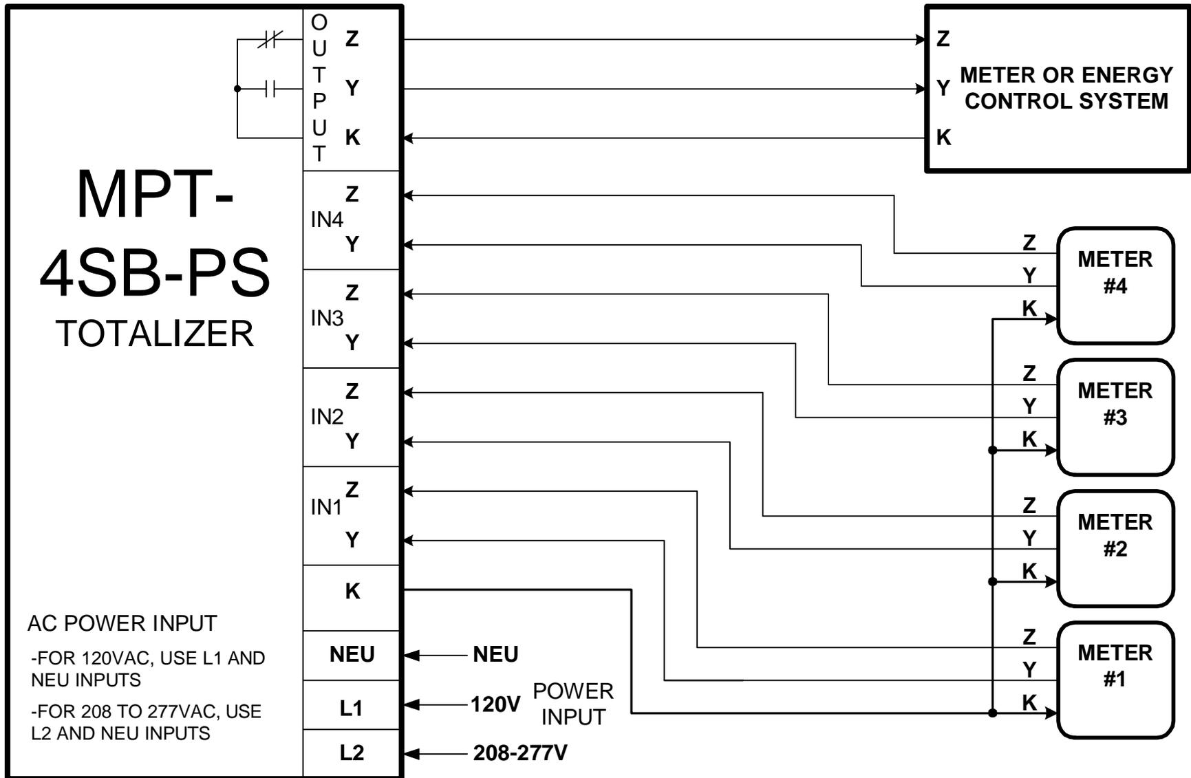
NOTE: A Sense Voltage of +13VDC is applied to the meters via the "Y" or "Z" leads from the MPT-4SB-PS. The "K" lead is the common return.
