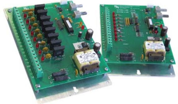
The OPL-8C system makes it possible to quickly implement an 8-channel optical pulse link with minimal effort. The system includes the power supply, wetting voltage, isolation relay and terminal block connectors making it possible to have a multichannel optical link up and running in minutes. The OPL-8C utilizes standard "ST" twist lock connectors and makes connections reliable, quick and easy. The multimode fiber optic cable is not included.
