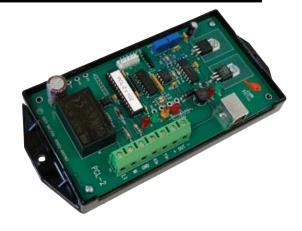
Upon receiving each pulse from the meter, the PCL-2's microcontroller calculates the instantaneous rate of usage based on the pulse rate and value, and updates the output to a current level between 4mA and 20mA. For example, suppose you have the full-scale output of the PCL-2 configured for 500kW. If a current demand of 250kW is calculated, the output would be adjusted to 12mA, the 50% midpoint between 4 and 20mA.
