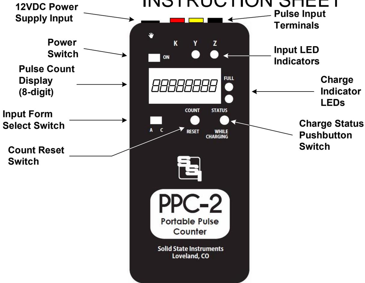
**GENERAL** - The PPC-2 is a battery-powered Portable Pulse Counter for KYZ pulse metering with Form A (2-Wire) or Form C (3-wire) pulse inputs. It can be used for water and gas meters as well as electric.
