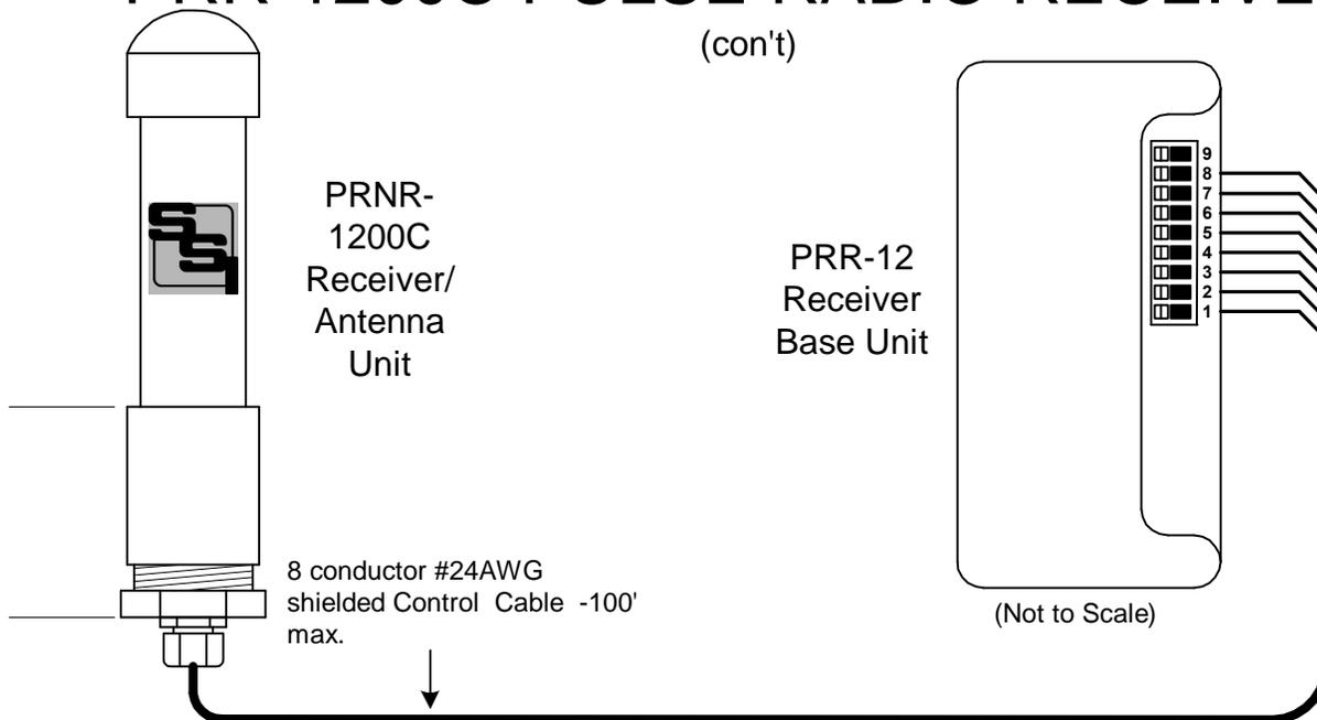
**POWER INPUT** - The PRR-1200C receives its power supply from the PRR-12 Receiver Base unit.
