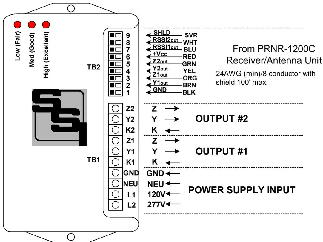
**GENERAL** - The PRR-12 serves as a base unit, and termination point for the PRNR-1200C receiver/antenna unit. It contains a power supply, output relays and all connection points for the receiver/antenna unit.
