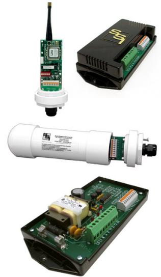
The PRL-1200 can transmit either 2 Form C (3-wire) pulses or 4 Form A (2-Wire) pulses. Approximately 4 pulses per second (Form C) while 2 Form A pulses are possible which should be more than acceptable for most pulse applications.
