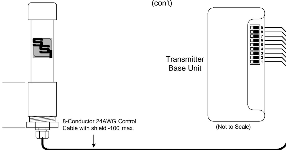
**POWER INPUT** - The PRT-900 receives its power supply from the PRT-2 Transmitter Base unit.
