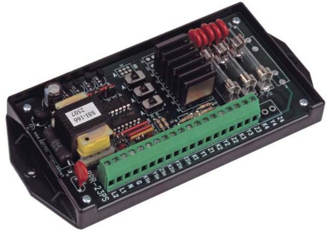
Typical applications include interfaces between utility metering devices and customer-owned energy control systems, demand recorder applications, or supervisory control systems (SCADA) interfaces.
