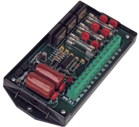
Typical applications include interfaces between utility metering devices and customer-owned energy control systems, demand recorders, or supervisory control systems (SCADA) interfaces.
