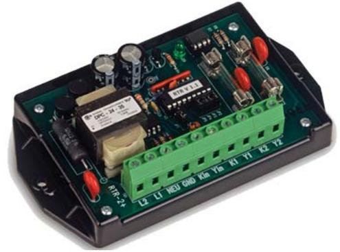
When the RTR-2+ relay is inserted in the two-conductor cable between the water or gas meter and the remote equipment, the RTR-2+ provides a replicated signal to the remote equipment, provides a separate isolated (dry contact) Form A contact for use with customer-owned monitoring equipment.
