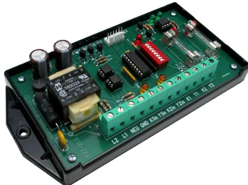
When the RTR-22+ relay is inserted in the two-conductor cable between the water or gas meter and the remote equipment, it provides a replicated signal to the remote equipment, provides a separate isolated (dry contact) Form A contact closure for use with customer-owned monitoring equipment.
