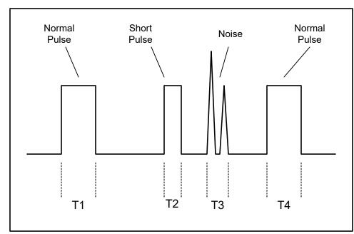
the time the input pulse is present. If the input pulse is present for less than the specified time (in milliseconds) as determined by the position of switches **S1.5, S1.6 and S1.7**, it is assumed to be noise. An input equal or longer in duration than the specified time is classified as a valid input and an output will occur. In the illustration to the left.
