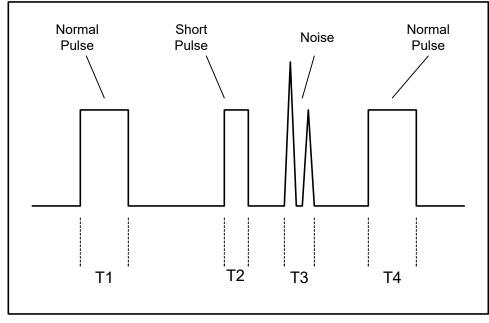
the time the input pulse is present. If the input pulse is present for less than the specified time (in milliseconds) as determined by the position of switches **S1.5** and **S1.6**, it is assumed to be noise. An input equal or longer in duration than the specified time is classified as a valid input and an output will occur. In the illustration to the left.
