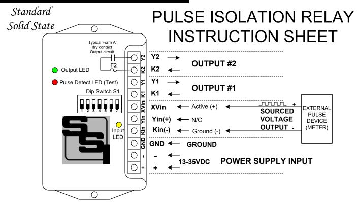
**<u>POWER INPUT</u>** - For a DC power supply of +13VDC to +37VDC, connect the "+" lead to the + terminal. Connect the "-" power supply lead to the - terminal. Connect the electrical system ground to the **GND** terminal. The unit must be grounded for proper operation.
