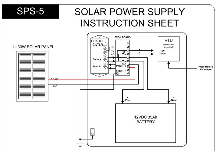
**MOUNTING POSITION** - The SPS-5 Enclosure must be mounted in an upright position so that the battery is placed on the <u>bottom</u> of the enclosure. Mount the solar panel using the metal mounting system provided to get the correct mounting angle pursuant to the instructions included in the mounting bracket kit. The solar panel mounting bracket is designed to attach to a pole or building. Solar Panel may not be shaded by trees or a building at any time.
