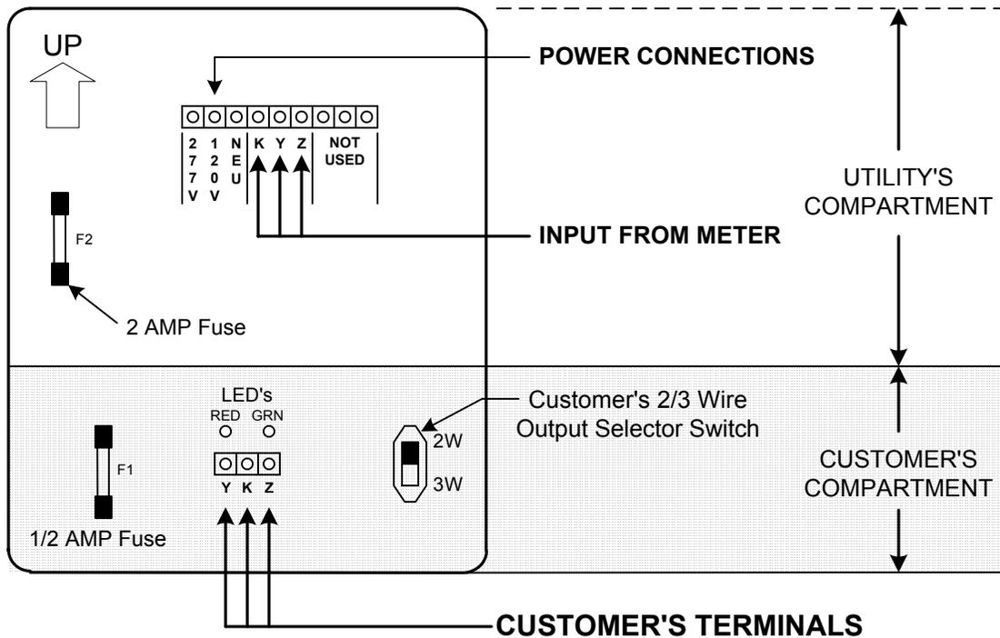
**MOUNTING POSITION** - Because the CIR-1A contains a mercury-wetted relay, it must be mounted in a vertical position to operate correctly.
