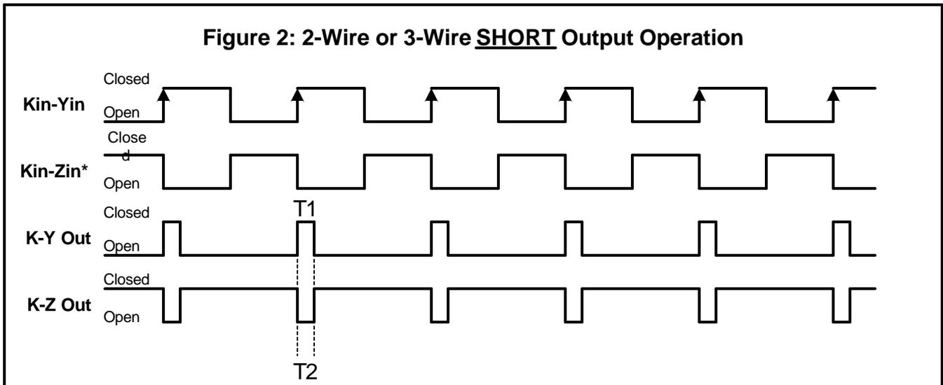
If the input pulse rate is greater than 9 pulses per second or if pulses of 100mS are too short for the receiving equipment, it is recommended that the LONG pulse output mode be used. Contact the factory for technical support at (888)272-9336.
