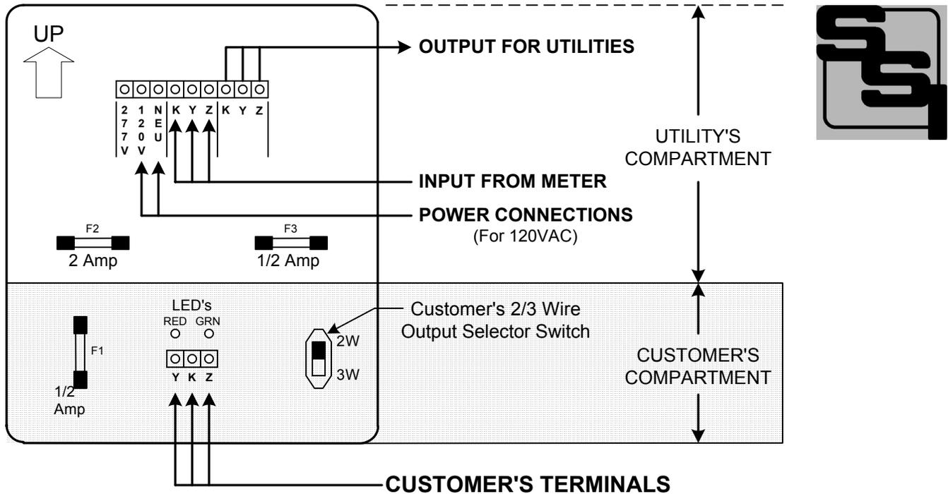
**MOUNTING POSITION** - Because the CIR-2A contains mercury-wetted relays, it must be mounted in a vertical position to operate correctly.
