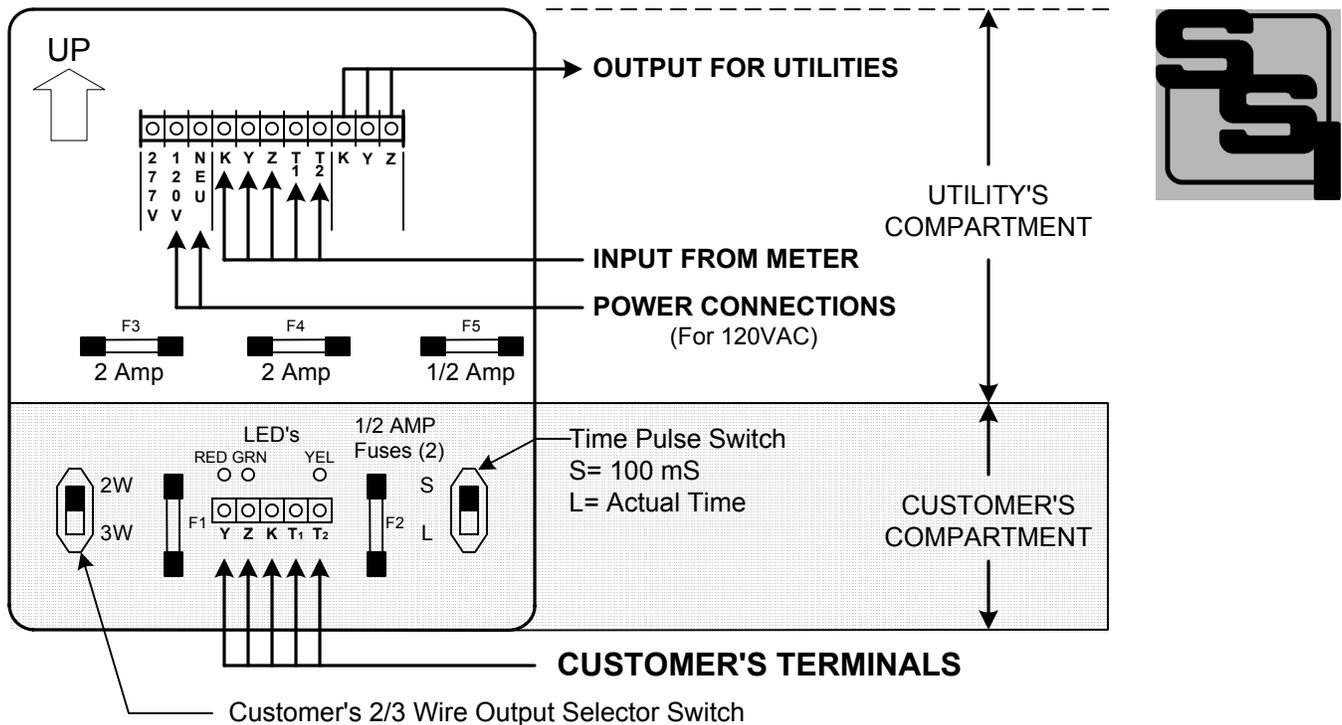
**MOUNTING POSITION** - Because the CIR-3A contains mercury-wetted relays, it must be mounted in a vertical position to operate correctly.
