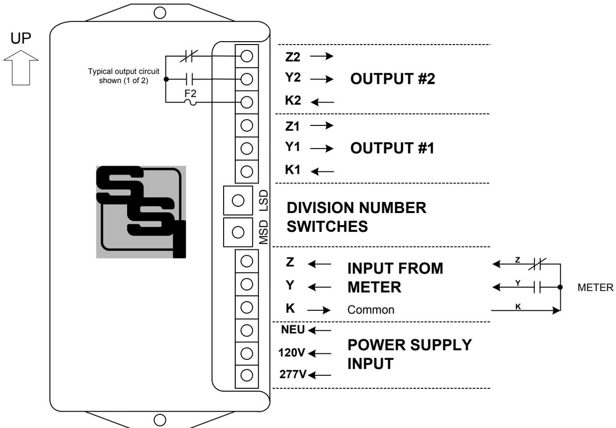
**MOUNTING POSITION** - Because the DPR-22 contains mercury-wetted relays, it must be mounted in a vertical position to operate correctly.
