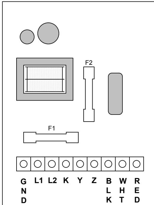
**POWER INPUT** - The GPR-1P should be powered by a 120VAC power source. Connect the "Hot" lead to L1 and the neutral lead to L2. Connect the ground wire to the GND terminal.
