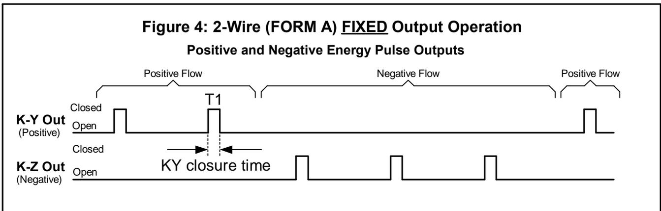
In Signed mode, with a Form A output mode selected, the K-Y output pulse represents positive (or kWh delivered) energy; K-Z output pulse represents negative (or kWh received) energy.
