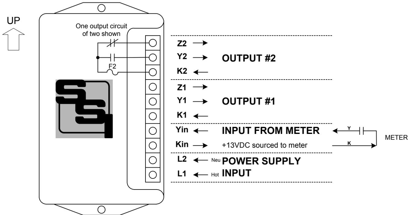
**MOUNTING POSITION** - Because the PIR-2C contains mercury-wetted relays, it must be mounted in a vertical position to operate correctly.
