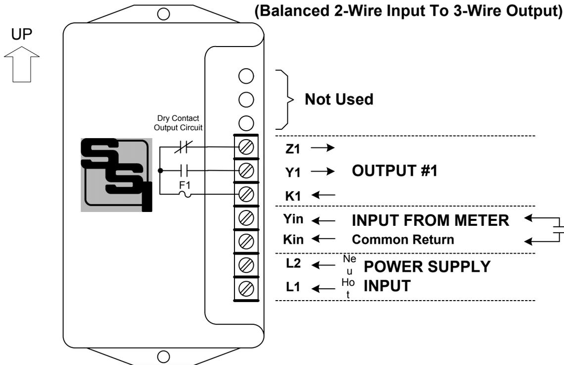
**MOUNTING POSITION** - Because the RPR-1LL-1 contains a mercury-wetted relay, it must be mounted in a vertical position to operate correctly.
