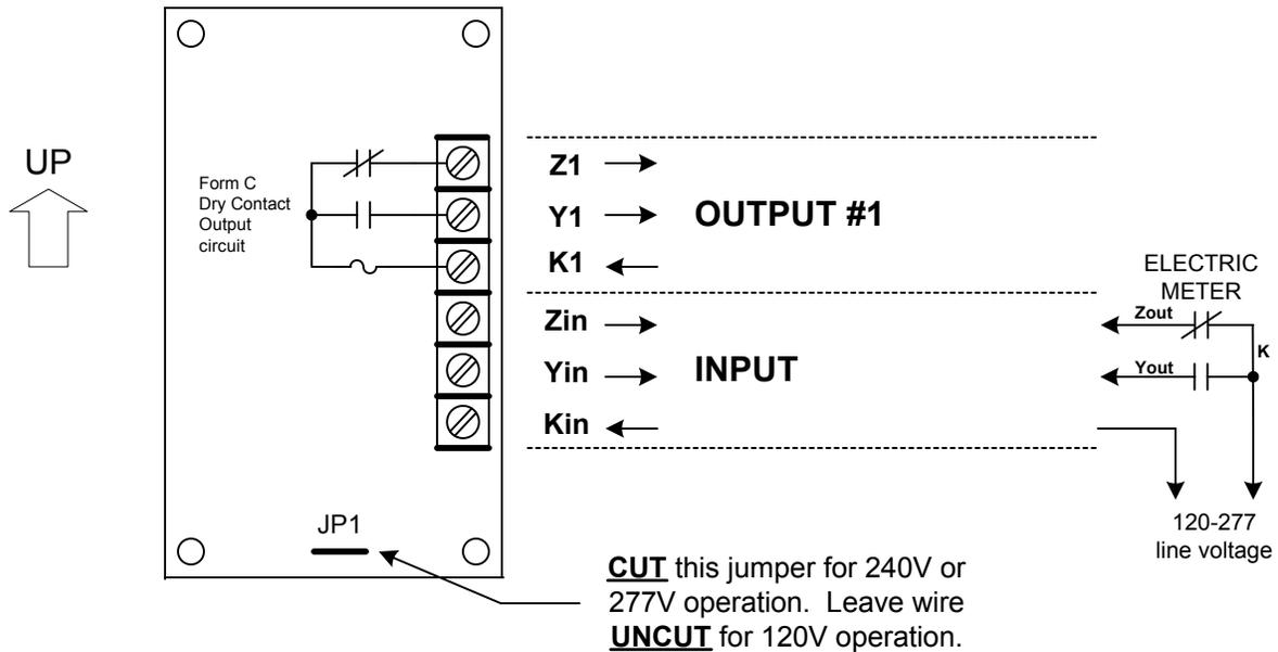
**MOUNTING POSITION** - Because the RPR-1 contains a mercury-wetted relay, it must be mounted in a vertical position to operate correctly.
