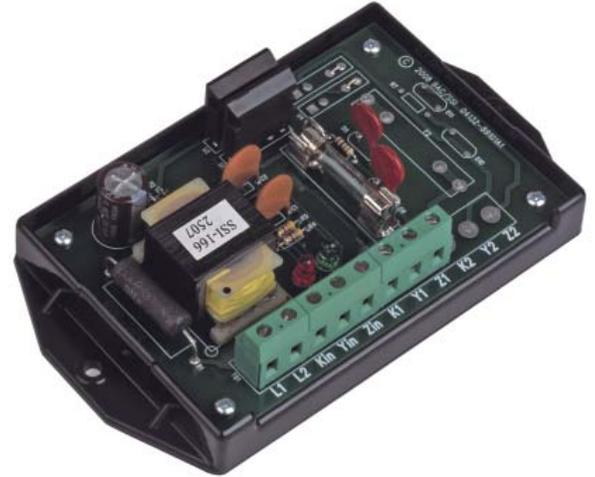
Typical applications include interfaces between utility metering devices and customer-owned energy control systems, demand recorder applications, and supervisory control systems (SCADA) interfaces.
