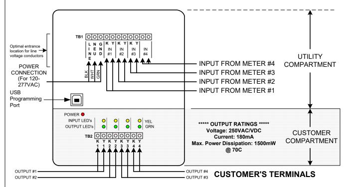
**ENCLOSURE** - The CIR-44 has a NEMA4X weatherproof and dustproof enclosure. The CIR-44 may be mounted in any position, but in general is most convenient and designed to be mounted with the hinge on the left side in the orientation shown above. Four mounting holes are provided.
