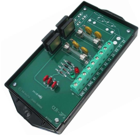
Applications include long distance pulse transmission interfaces up to 2-4 miles between utility metering devices and customer-owned energy control systems, demand recorders, or supervisory control (SCADA) systems.
