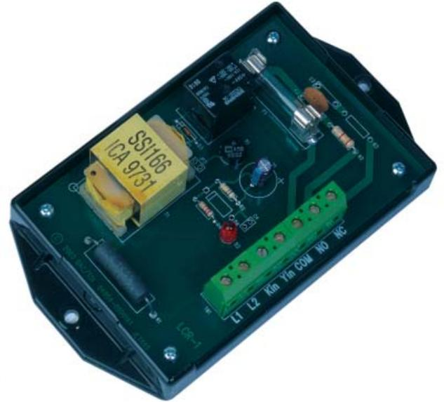
The LCR-1 has a built-in low voltage transformer isolated power supply and may be used with meters having mechanical output contacts (relays), or high or low voltage semiconductor outputs.
