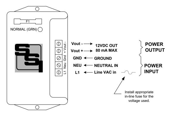
**GENERAL** - The MPS-2-12 is a power supply for KYZ Pulse Metering. It is designed to provide a "wetting" or sense voltage to the "K" terminal of a KYZ pulse initiator or an isolated dry-contact output. This sense voltage is switched on and off as the KY and KZ terminals are closed to source this voltage to another "downstream" device which does not supply its own wetting voltage.
