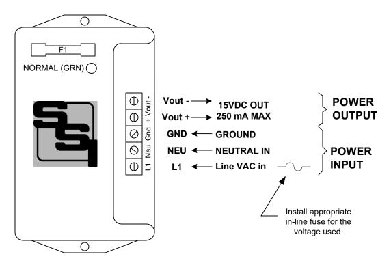
**GENERAL** - The MPS-2-15 is a power supply for KYZ Pulse Metering. It is designed to provide a "wetting" or sense voltage to the "K" terminal of a KYZ pulse initiator or an isolated dry-contact output. This sense voltage is switched on and off as the KY and KZ terminals are closed to source this voltage to another "downstream" device which does not supply its own wetting voltage.
