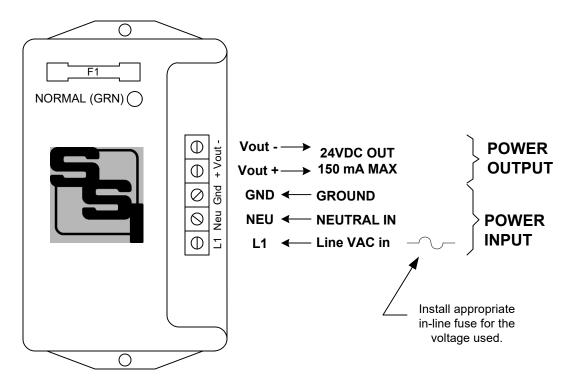
**GENERAL** - The MPS-2-24 is a power supply for KYZ Pulse Metering. It is designed to provide a "wetting" or sense voltage to the "K" terminal of a KYZ pulse initiator or an isolated dry-contact output. This sense voltage is switched on and off as the KY and KZ terminals are closed to source this voltage to another "downstream" device which does not supply its own wetting voltage.
