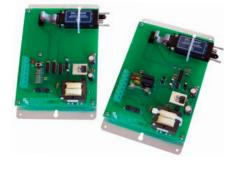
be used as a Form A (2-wire) or a Form C (3-wire) depending on the transmitter's input configuration selection. This system makes it possible to quickly implement an optical pulse link with minimal effort and includes all power supplies, wetting voltages, isolation relays and connectors.
