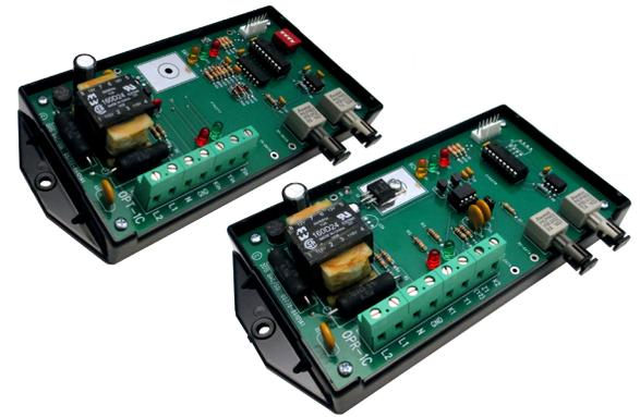
Each system consists of an OPT-1C transmitter and an OPR-1C receiver. The OPT-1C transmitter is designed to receive pulses from an electric meter's KYZ pulse initiator. Pulses are conditioned, encoded and sent by fiber optic cable to an OPR-1C receiver where the pulse information is decoded, validated and implemented into the correct pulse state. The OPT-1C transmitter and OPR-1C receiver must be paired and cannot be used independently. Fiber optic cable not included.
