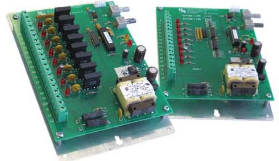
The OPL-4C system makes it possible to quickly implement a 4-channel optical pulse link with minimal effort. The system includes the power supply, wetting voltage, isolation relay and terminal block connectors making it possible to have a multichannel optical link up and running in minutes. The OPL-4C utilizes standard "ST" twist lock connectors and makes connections reliable, quick and easy. The multimode fiber optic cable is not included.
