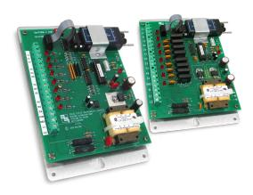
The OPL-8B system makes it possible to quickly implement an 8-channel optical pulse link with minimal effort. The system includes the power supplies, wetting voltage, isolation relays, and terminal block connectors making it possible to have a multichannel optical link up and running in minutes. The OPL-8B utilizes standard "ST" twist lock connectors and makes connections reliable, quick and easy. The fiber optic cable is not included.
