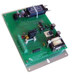
as a Form A (2-wire) or a Form C (3-wire) depending on the transmitter's input configuration selection. An OPR-1B receiver requires an OPT-1B transmitter.
