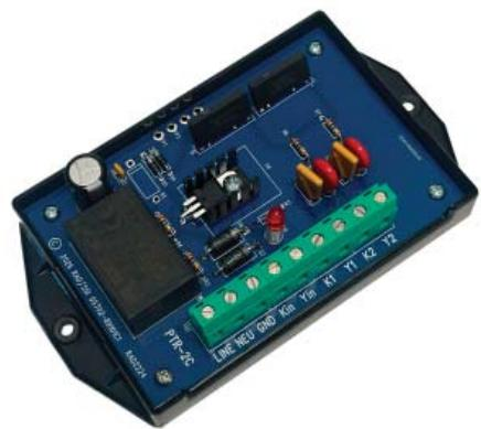
The PTR-2C is intended to be located at the location of the receiving equipment – usually a customer-owned energy management system. It acts primarily to protect the customer equipment from large transients that could be coupled into long wire runs between it and the electric meter. Transients which are coupled into the wire loop between the originating pulse output and the PTR-2C are contained within the loop and suppressed by means of heavy-duty transient suppression devices.
