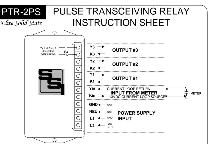
**MOUNTING POSITION** - The PTR-2PS may be mounted in any position.
